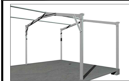
2A FIRST & SECOND PORTAL FRAME ASSEMBLY REFER 2C FOR TEMPORARY BRACING LOCATION
